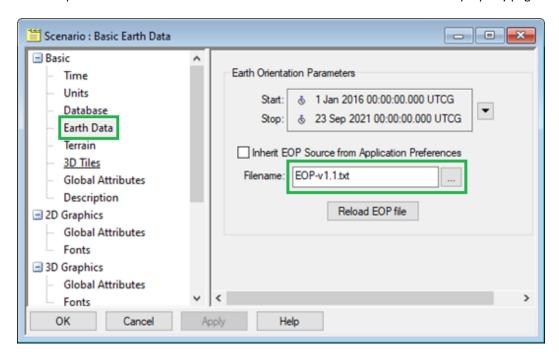
The EOP file in the ODTK application is specified via the object properties on the scenario, as shown:
