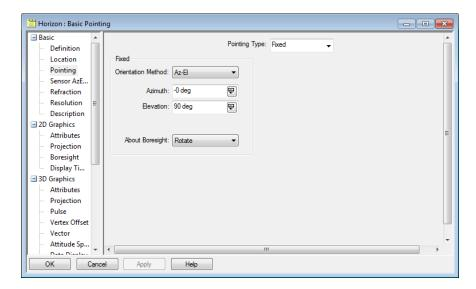
The code that implements these choices in CreateSensors(), except for the names of the interfaces, should look familiar by now. The important thing to note is that after you use the IAgOrientationAzEI interface to set the Elevation and AboutBoresight properties, it all must be assigned back into the Orientation property of the interface representing the Fixed pointing type (using the IAgOrientation interface's Assign() method).
