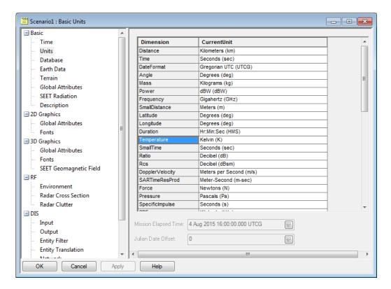
In the Object Model, you can use the SetCurrentUnit() method to set the any of these units explicitly. Here you will use it to change the preferred unit for Temperature from Kelvin (K) to degrees Celsius (degC).
