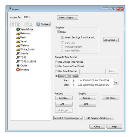
In the illustration, the Access tool has been launched from the ERS1 satellite – the 'from' object – and the area target has been selected as the 'to' object. Access is computed when someone clicks the Compute button or selects one of the report, graph or display options.
