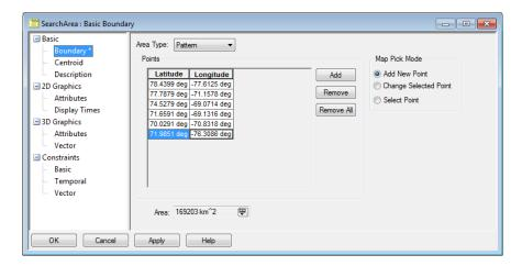
In this example, the Pattern Area Type is selected to define the boundary (the other option is Ellipse). Latitude and longitude values for boundary points are added to a list, and the boundary is created by drawing Great Arc lines between those points.
