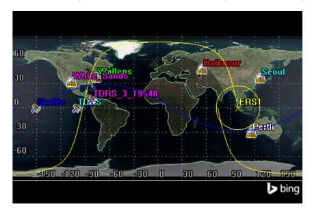
To see the effect of AccessDisplayIntervals(), create a new scenario, and then select Create Facilities, Create Satellites, Create Sensors and Access Display Intervals. Animate the scenario and observe how the ERS1 satellite and its sensors disappear from view in the 2D and 3D windows except when there is access to a facility.
