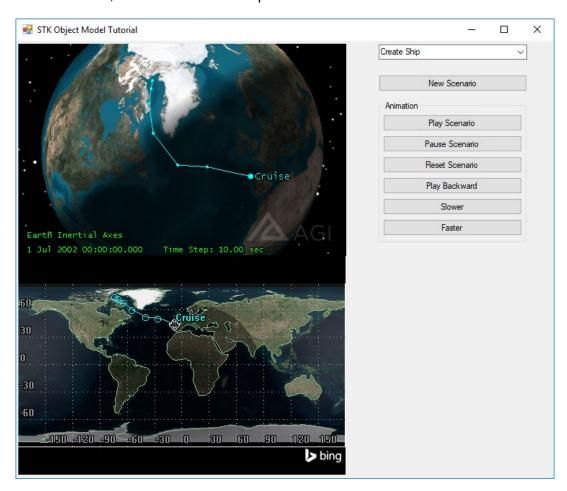
Here you can use the mouse to rotate and zoom in on the 3D view, taking advantage of functionality that became available as soon as you dragged the AGI Globe Control onto the form.
