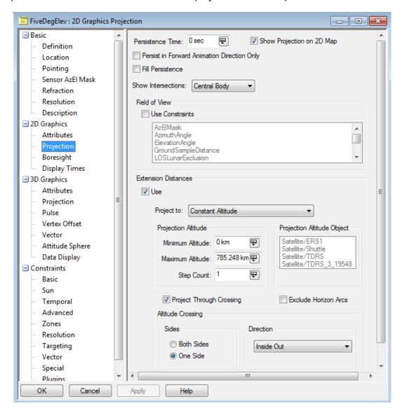
The LimitSensorVisibility method uses the IAgSnProjDisplayDistance interface to implement the above settings, including the selection of Constant Altitude as the 'Project to' option and the settings for minimum and maximum altitude and step count.
