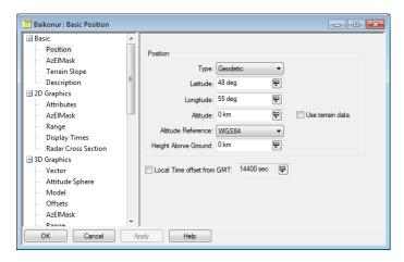
In the above example, the facility is defined using the Geodetic position type, make sure the terrain is turned off.
