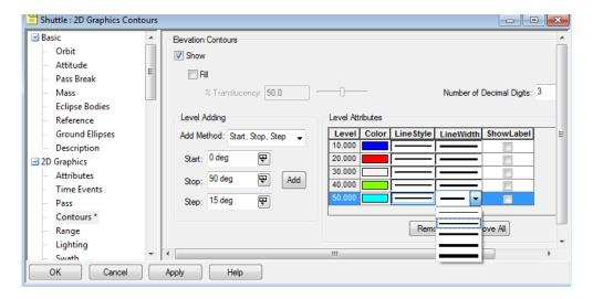
In the above example, you have selected Start, Stop, Step as the Add Method and set the corresponding values to define 6 contour levels spaced 10 degrees apart. Use the Remove All button to get rid of any existing contour graphics, and then click Add to populate the Level Attributes list with our newly defined contours. After increasing the LineWidth and disabling the ShowLabel option of each contour, select the Show checkbox to display the contours.
