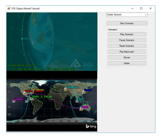
The FiveDegElev sensor, attached to the Wallops facility, is of the Complex Conic Sensor Type. The outer cone half-angle is set to 85 deg to limit the sensor's visibility to objects at an elevation of 5 degrees or higher:
