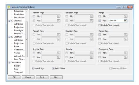
The AccessConstraintsRange() method uses properties exposed by the IAgAccessCnstrMinMax interface to enable a maximum range constraint and set its value. The interface is initialized by calling the AddConstraint method of the IAgAccessConstraintCollection interface (made available via the sensor's AccessConstraints property), which returns information on the selected constraint type.
