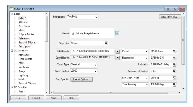
In the above example, the satellite is propagated using the TwoBody propagator, and the orbit is defined using Classical (Keplerian) elements, with Period and Eccentricity defining the orbit's size and shape; Inclination, Argument of Perigee and Longitude of Ascending Node defining its orientation; and True Anomaly defining the location of the satellite in the orbit.
