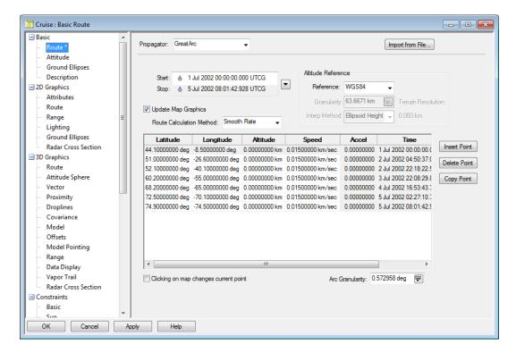
Each row in the table represents a waypoint, with the specified latitude, longitude, altitude, speed, acceleration, time and turn radius. You may notice that two of the columns – those for acceleration and time – are grayed out. Those values are read-only, because the Route Calculation Method is set to Smooth Rate, which derives acceleration and time from speed and position.
