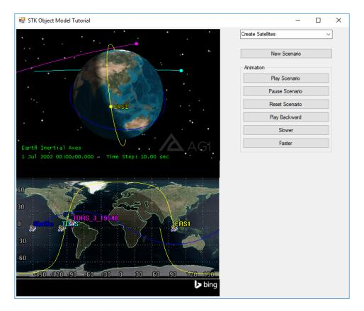
Another method in this section, ModifyShuttleDisplay(), lets us tweak and enhance the 2D Graphics properties of the Shuttle. After using the IAgVeGfxAttributesOrbit interface to change the satellite's marker and line style, the method draws elevation contours around it.
