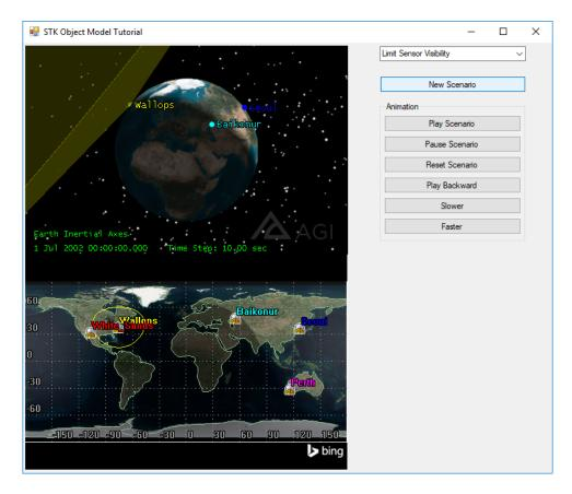
You can further restrict the sensor's field of view by decreasing the outer cone half angle. For example, reduce it to 75 deg to impose a 15-degree elevation requirement.
