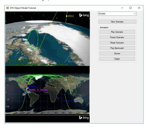
To remove access computations and graphics, the RemoveAccess() method uses the IAgStkAccess interface's method of the same name. To test it, update the SelectedIndexChanged() method, set up the access computation described above, and then select RemoveAccess from the combo box.
