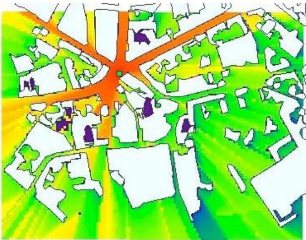
Figure 7. (U) Real Time Path Loss, Milan, Italy
