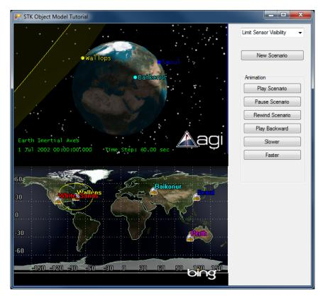
You can further restrict the sensor's field of view by decreasing the outer cone half angle. For example, reduce it to 75 deg to impose a 15 degree elevation requirement.
