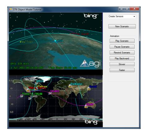
The FiveDegElev sensor, attached to the Wallops facility, is of the Complex Conic Sensor Type. The outer cone half-angle is set to 85 deg to limit the sensor's visibility to objects at an elevation of 5 degrees or higher:
